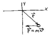
D. 1. Applying the right hand rule to these vectors shows that  $\vec{L} = \vec{r} \times \vec{p}$  points in the <u>negative z direction</u>. (Draw the vectors with their tails together. Then, wrap your fingers around the vertex of the angle, pointing from the first vector toward the
