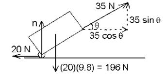
A constant speed means the acceleration is zero. If you put zero acceleration into Newton's second law, you get  $\Sigma F_x = 0$  and  $\Sigma F_y = 0$ .
